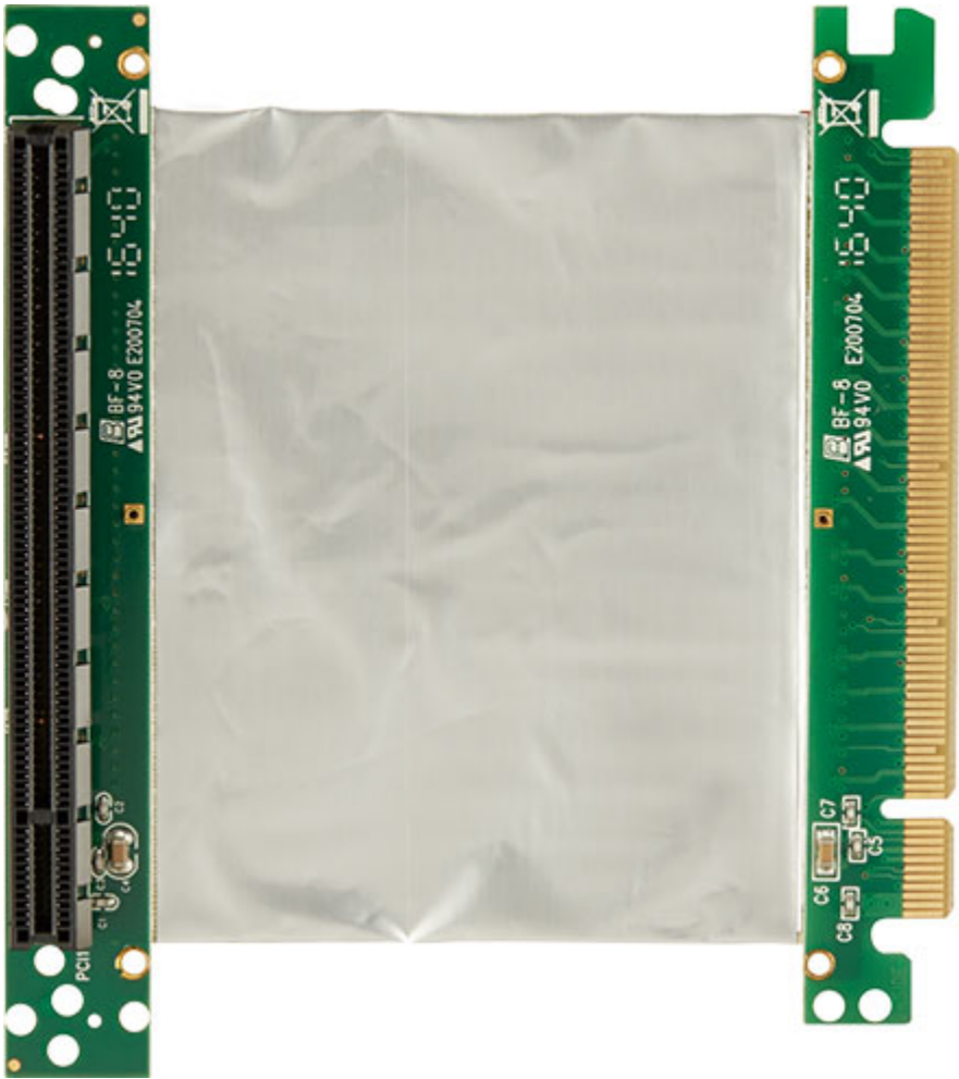
PClex16 to PClex16 riser card, L=100 mm
